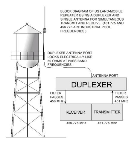
Caption: An example figure of a duplexer used in a US Land-Mobile Repeater for simultaneous transmit and receive.
