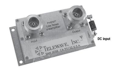
Each preamplifier is housed in a rugged, custom-made, RF-tight aluminum enclosure. The DC input is reverse polarity protected, and equipped with a high-pass filter to eliminate RFI.
